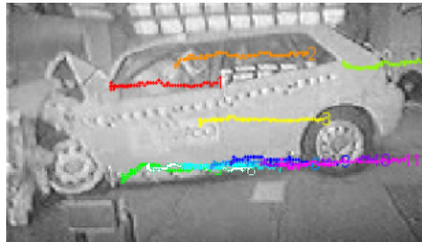
Figure 16 Trajectories of points on a car body during a crash test
