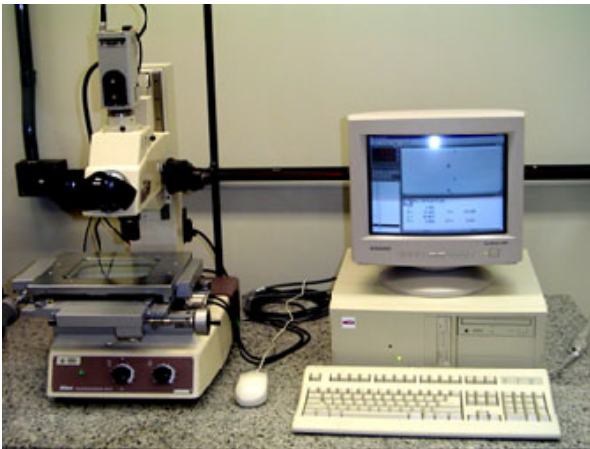
Figure 5: NIKON MM40 optical microscope (resolution = 1 \mu\text{m} ) used to measure the electrode edge radius growth
